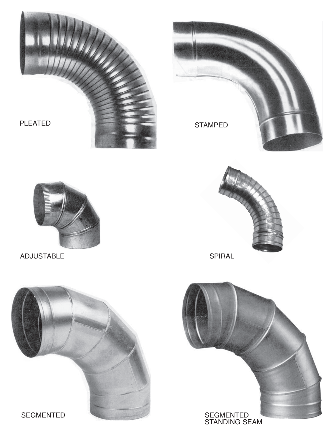
FIGURE 3-4 ROUND DUCT ELBOWS
